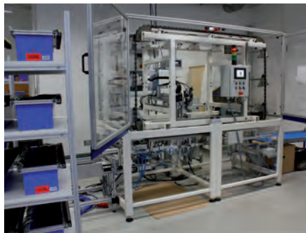
Automated filling of 2K-epoxy resin at the moulding station
