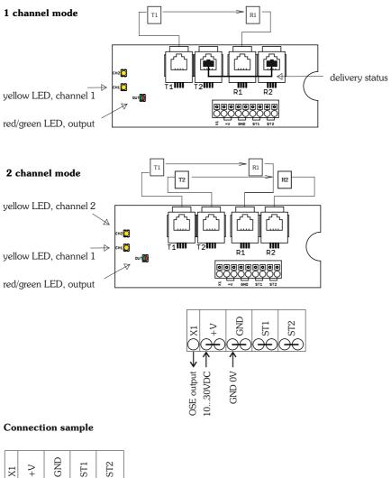
PLUS or MINUS for safety circuit pass door/slack rope switch
